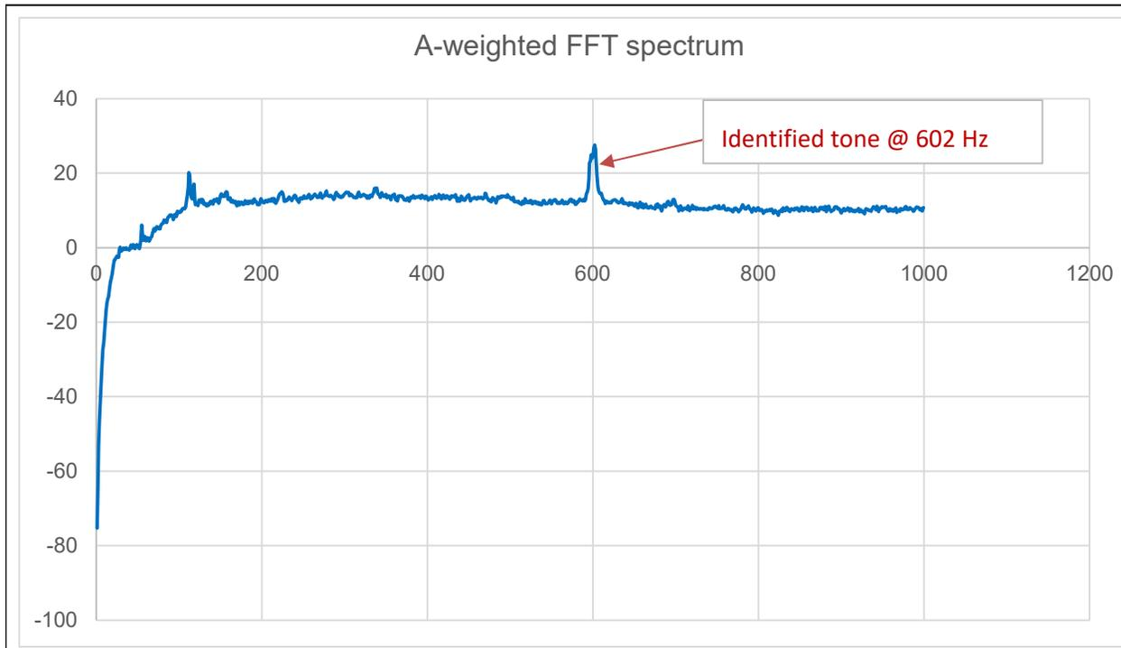
**FIGURE F3: FFT PLOT WITH AN IDENTIFIED TONE (A VALID INTERVAL FROM PHASE 2B AT 2019-04-14 02:10)**
