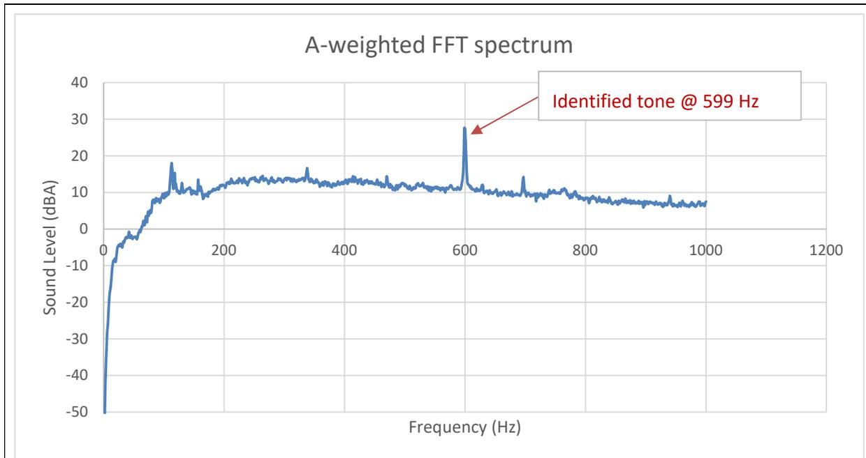
**FIGURE F1: FFT PLOT WITH AN IDENTIFIED TONE (A VALID INTERVAL FROM PHASE 2B AT 2020-05-03 21:00)**
