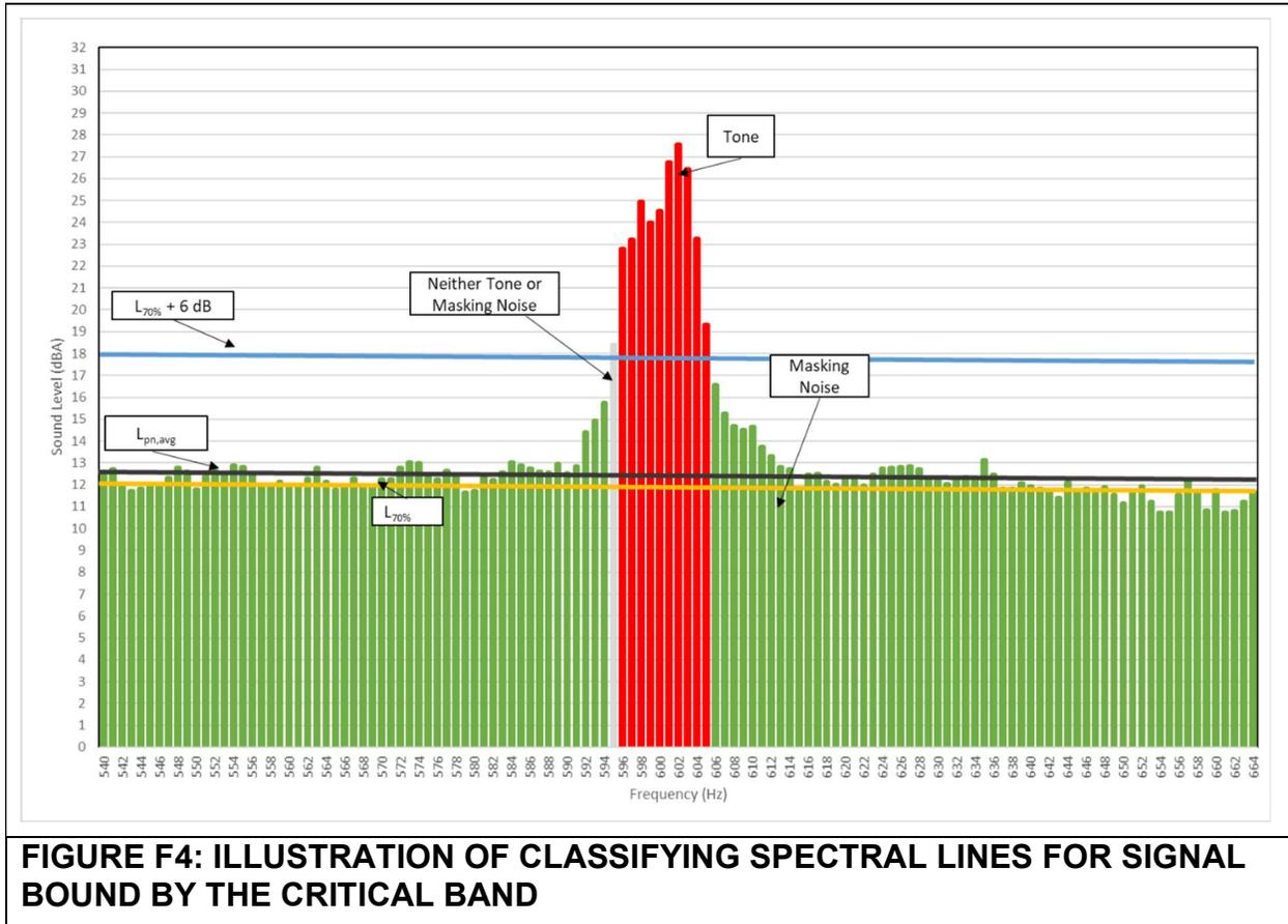
**FIGURE F4: ILLUSTRATION OF CLASSIFYING SPECTRAL LINES FOR SIGNAL BOUND BY THE CRITICAL BAND**
