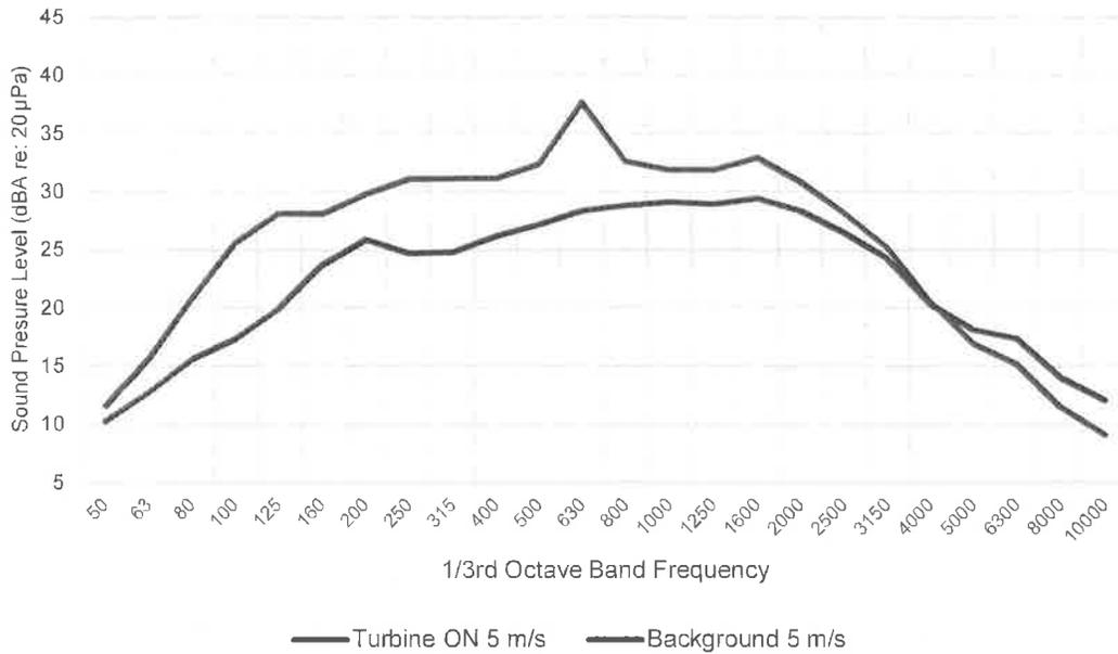
Evident in Figure 4 is an elevated sound level present in the immission measurement data at the same 630Hz 1/3<sup>rd</sup> octave band observed at the turbine in the IEC 61400-11 test. The sound level in this frequency band is the highest contributor to the overall sound level, with a measured impact over 5 dB higher than the next highest frequency band. Based on the sound levels measured at the receptor, the acoustic issue of most importance is the 600Hz tone from the wind turbine gearbox.
