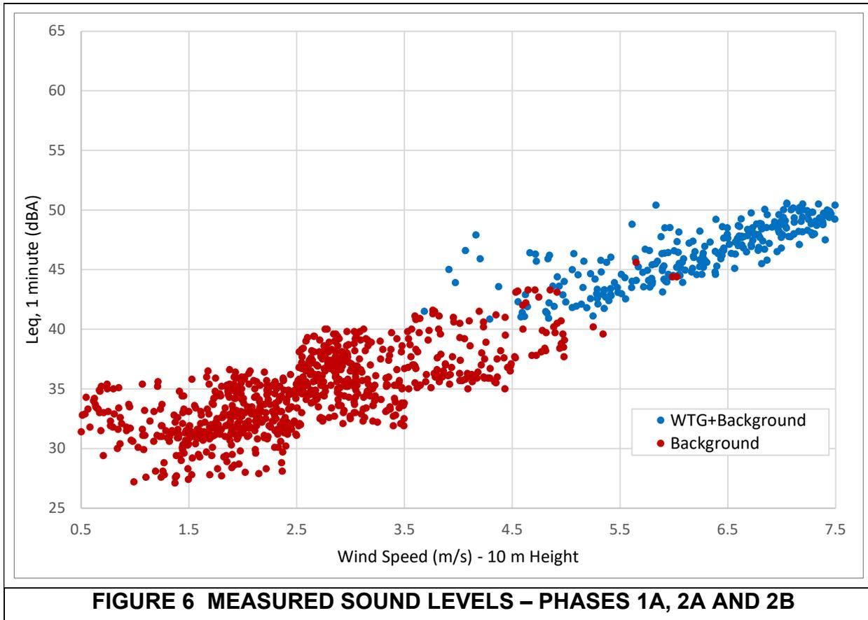
As shown in Table 8, a sufficient number of valid data points were retained at the 5 m/s, 6m/s and 7 m/s wind speed bins for the turbine on scenario. For the turbine parked scenario, a sufficient number of valid data intervals/points were retained at the wind speed bins from 1 m/s to 6 m/s in accordance with the Part E of the MECP protocol.
