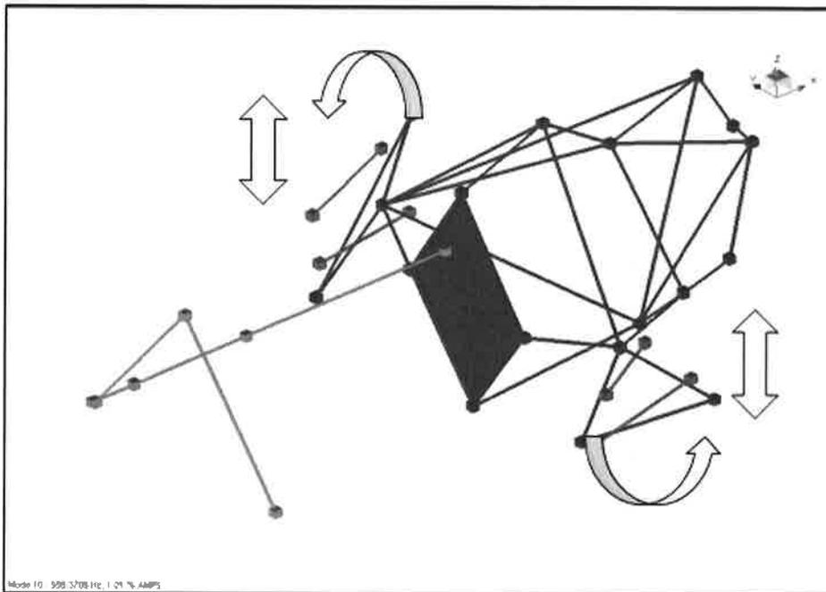
In a First Step we checked to bring 2x TMD to both side of the torque arms at the back side of PINS. This reduce the torsional mode but not the tone in the WTG airborne noise. The flapping stays but changed a little by amplifying the front side Pin.
