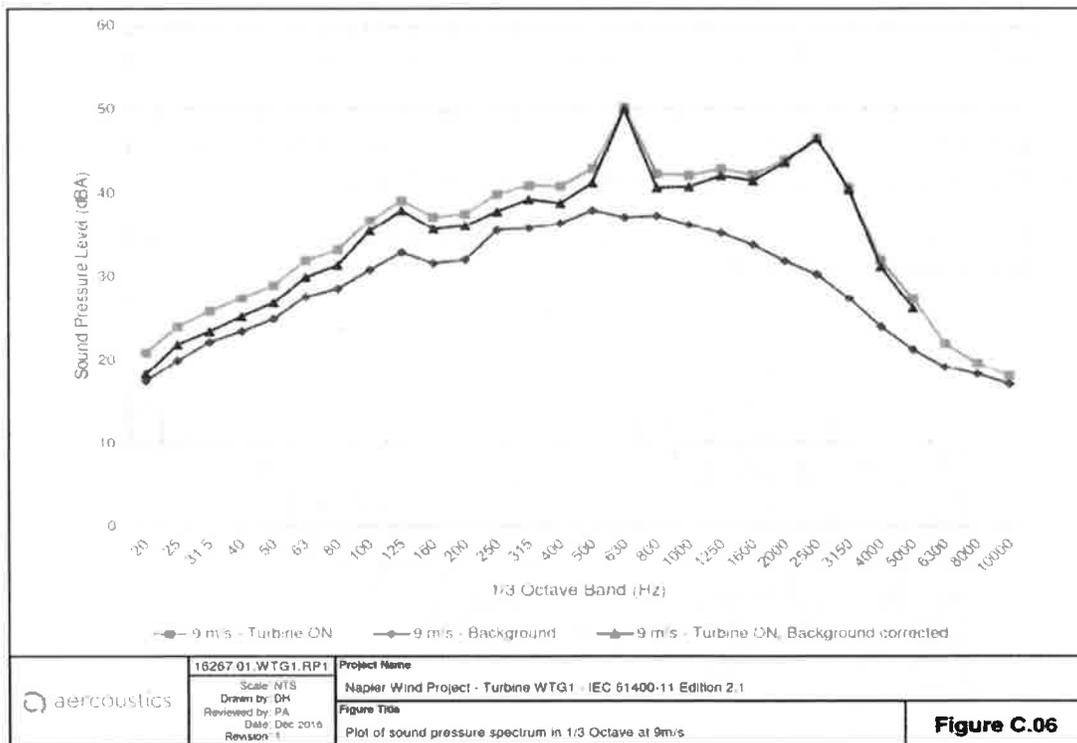
From Figure 2, it is apparent that the elevated sound levels at the 630Hz octave band is the single biggest contributor to the overall sound level from the turbine.
