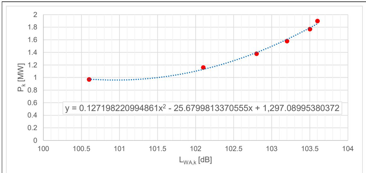
**FIGURE D1: RELATIONSHIP BETWEEN MEASURED ELECTRICAL POWER OUTPUT AND MEASURED SOUND EMISSION LEVEL**
